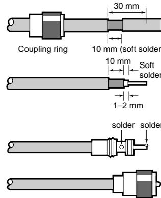
① Slide the coupling ring down. Strip the cable jacket and soft solder.
