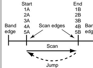
5 pairs of scan edges are available and scans 1A–1B (P1), 2A–2B (P2), 3A–3B (P3), 4A–4B (P4), 5A–5B (P5).
