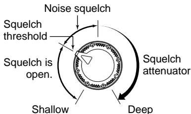
**NOTE:** The squelch attenuator functions even when the monitor function is in use. Thus set **[SQL]** control within 10 to 12 o'clock position is recommended when using the monitor function.
